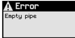
In case of any error, the error message is displayed on the display for approx. 1 to 5 seconds. The same error message can be read by computer using RS232 or RS485 (command IER?).
