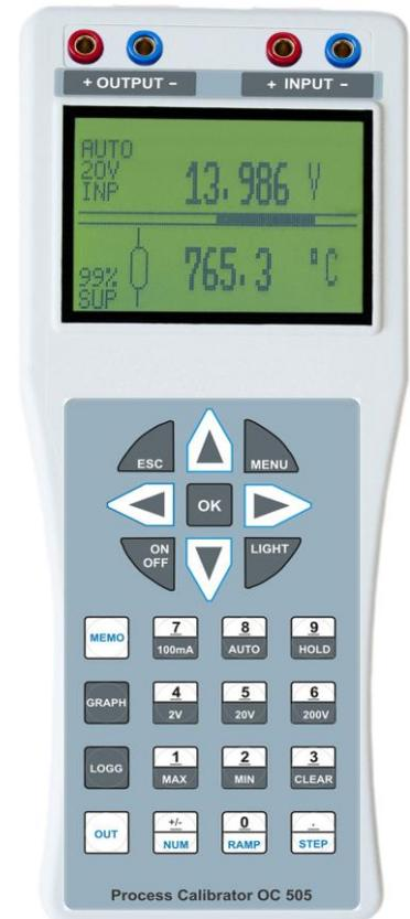
**M505** is a Calibrator-Multimeter for generation of Currents 0-22mA Sink or Source and Voltages to 25VDC. External voltages  $\pm 2V$ ,  $\pm 20V$  and  $\pm 200VDC$  (firm ranges or auto ranging) and Currents to  $\pm 100mA$  can be measured simultaneously and shown at the display.
