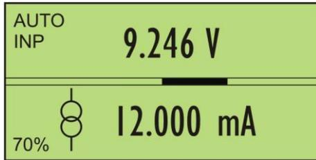
**MULTIMETER** measured input voltage in automatic range.
