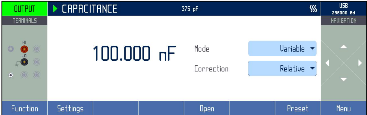
Figure 29 Capacitance screen with OPEN position
