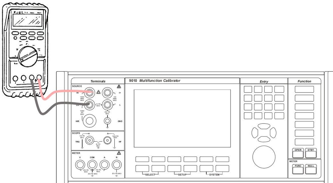
Obr. 25 Kalibrace kapacity
