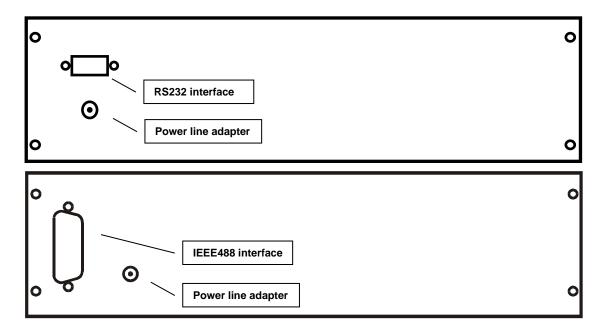
On the rear panel there are located power supply connector, interface RS-232 connector (optionally IEEE488 connector) and serial number plate.
