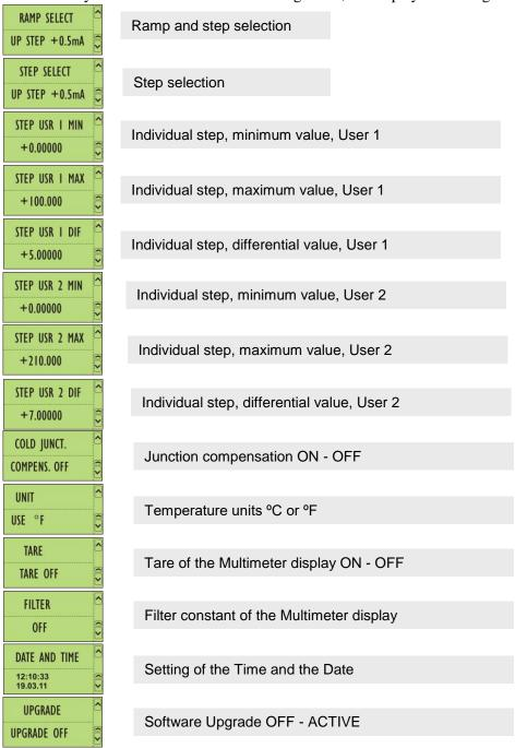
With **ESC** one return step in Menu is possible. By pressing **ESC** three times, the display returns into the measuring mode.
