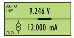
MULTIMETER measured input voltage in automatic range.
