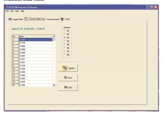
Number Eight memory slots for fast signals at the multimeter input. Each Transient contains
