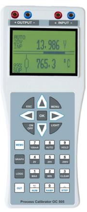
Further Functions contain generation of calibration mV Signals, Thermo voltages of DIN Thermocouples and RTD Resistors and simulation of true resistors.
