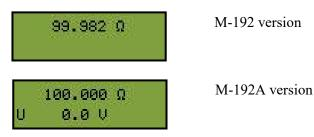
In the upper row generated resistance in  $[\Omega]$  is displayed. In the lower row mesaured voltage connected to the output terminals (M-192A only) is displayed.
