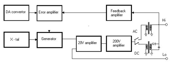
In 1000 V AC mode, the output of 200 V amplifier is transformed and led to the output terminals. The output voltage is sensed, rectified and compared to reference DC voltage provided by the DA converter. error value controls the amplitude of the generator's output so that there is correct voltage at the output terminals. In 1000 V DC mode,  $12~\rm kHz$  signal is transformed, rectified, filtered and led to the output terminals. The output voltage is sensed equally to  $1000~\rm V$  AC mode.
