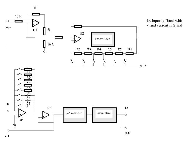
Hi and Lo are calibrator's output terminals. The stage including U1 operating amplifier converts voltage to current. U2 is a separation amplifier. R1 to R5 and C1 to C3 are range impedance. DA converter has 0 to  $\pm$ 1 and 0 to  $\pm$ 1 conversion ration and allows the simulation of resistance and capacitance values different from the range impedances. The output stage increases the permitted current load of the output.
