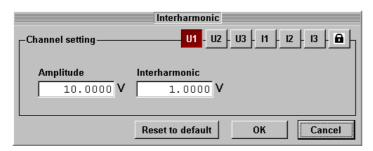
The interharmonic window allows setting of interharmonic component in the output signal. Selection of calibrator's output is described in previous paragraph (Harmonic window).
