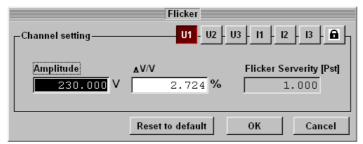
The Flicker window allows setting of the output signal amplitude and modulation. Selection of calibrator's channels is described in previous paragraph.
