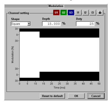
The modulation window allows setting modulation of the output signal. Selection of calibrator's output is described in previous paragraph (Harmonic window).
