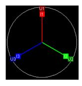
In the upper right corner is displayed vector diagram. There are displayed or current (I1, I2, I3) and voltage (U1, U2, U3) outputs. North pointing vector (position on the twelve o'clock) shows angle  $0^{\circ}$ . South pointing vector (position on the six o'clock) shows angle  $180^{\circ}$ . The picture shows outputs I1, U1 (angle  $0^{\circ}$ ), outputs I2, U2 (angle  $120^{\circ}$ ) and outputs I3, U3 (angle  $240^{\circ}$ ).
