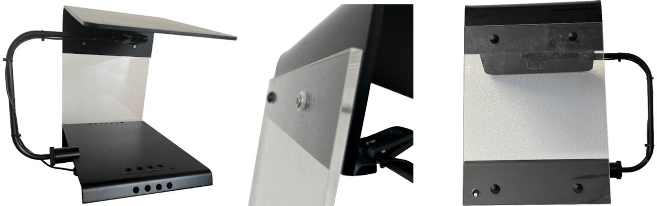
Next up, slide the camera arm jaw onto the base plate, position the arm so that the camera is approximately 15 cm or 6 inches away from the DUT display and secure it in place by tightening the jaw bolt (using attached hex key) and toothed wheel on the side of the jaw. Recommended jaw position is around  $\frac{1}{4}$  of the base plate length
