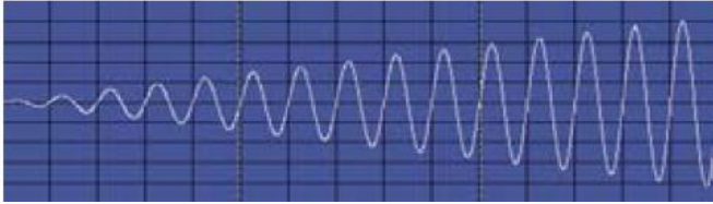
Output voltage waveform based on voltage of slew rate setting
