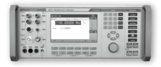
Advancing from previous M14x calibrator series, 9010+ can now calibrate even 6½ digit DMMs, 1CHz o-scopes, power analyzers, 1.5 kV insulation testers, clamp meters and more. Fixed resistor and capacitor series allows for calibration of more accurate ohm meters than competitive calibrators would. Builtin multimeter for transducer and external sensor calibration (strain gauge, pressure, torsion, strength, etc.) remains available in 9010 series too.
