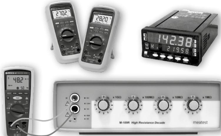
Calibration and verification of resistance meters with test voltage up to 5 kVDC
