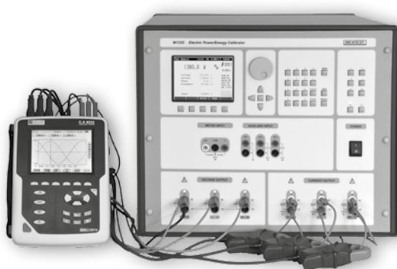
Clampmeter calibration with 151-25 Current Coil
