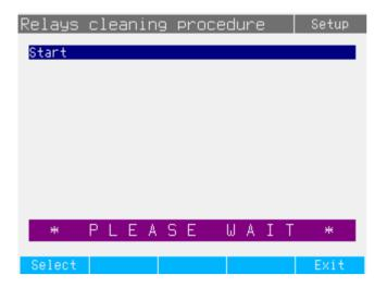
The procedure lasts about 15 second. During procedure 5320A cannot be operated.
