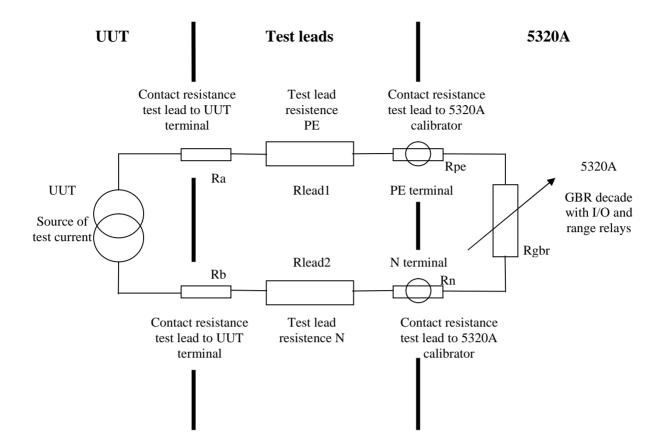
The resistances shown between the 5320A and the UUT are often referred to as parasitic resistances. This application note describes how to compensate for the parasitic resistors, to properly test the UUT
