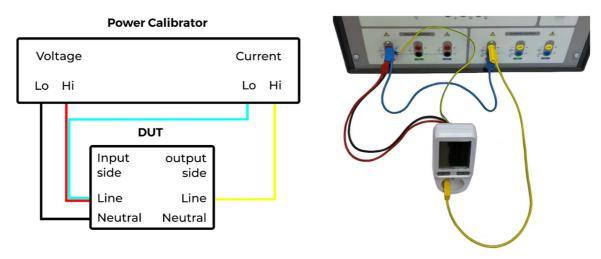
DUT ground pin can be optionally grounded through Voltage-LO terminal of the calibrator provided the voltage output is internally grounded (V-GND ON).
