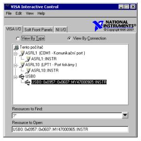
All the connected instruments and their identification string are shown in this panel. In the picture you can see the HP34410 instrument connected to the USB bus.
