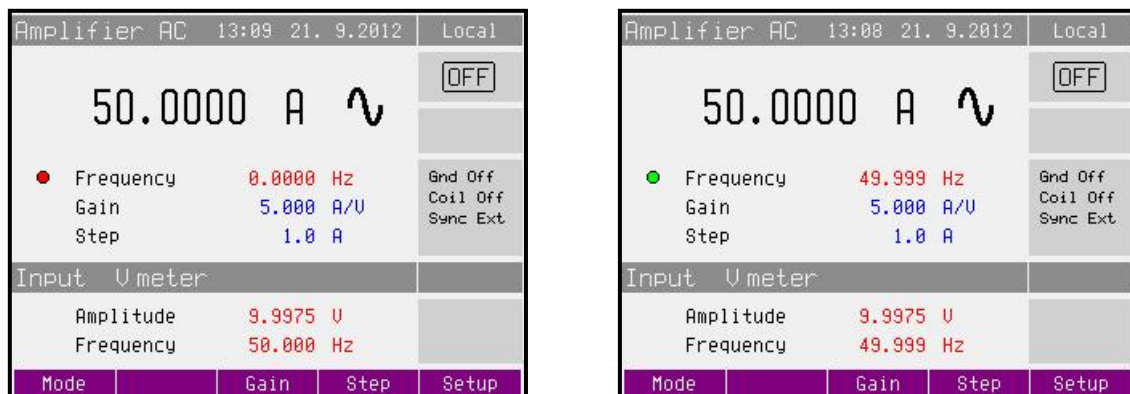
Figure 7 Transconductance AMPLIFIER - frequency and phase synchronization
