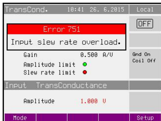
Figure 6 Transconductance AMPLIFIER – Slew rate and high amplitude
