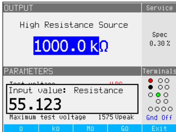
Figure 1. Keypad Entry Display
