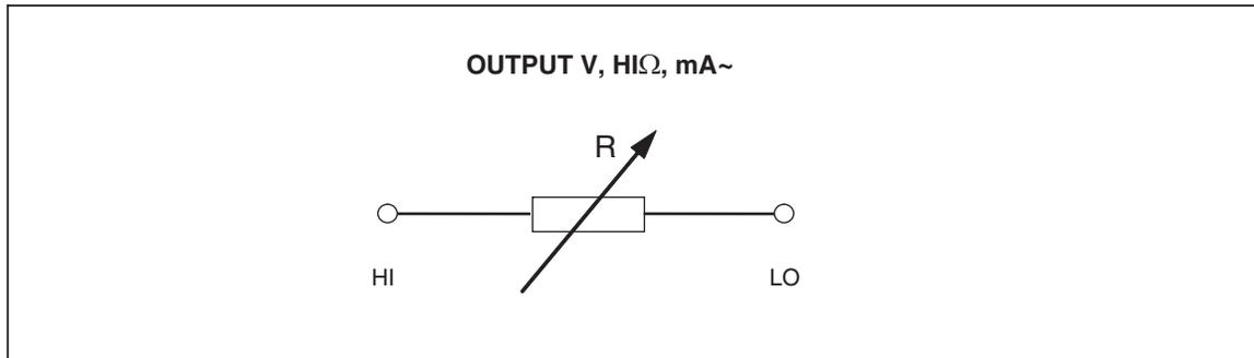
Figure 4. Simplified High Resistance Source Scheme
